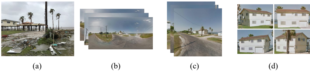
Figure 1. Detection of a house from Google Street View: (a) post-disaster building images collected after Hurricane Harvey in 2017, (b) 360° panorama images downloaded from Google Street View, (c) 2D images projected from the panorama images using the optimal project directions, and (d) house images detected from the images in (c).
