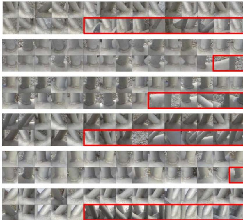
Figure 4. Examples of ROIs that have been localized and classified from the set of test images: Each set of 30 localized ROIs corresponds to Welds 1 to 6 (from top to bottom). A maximum of 10 negatively classified ROIs, are positioned at the end of the set (marked with a red box). The rest are classified as positive.
