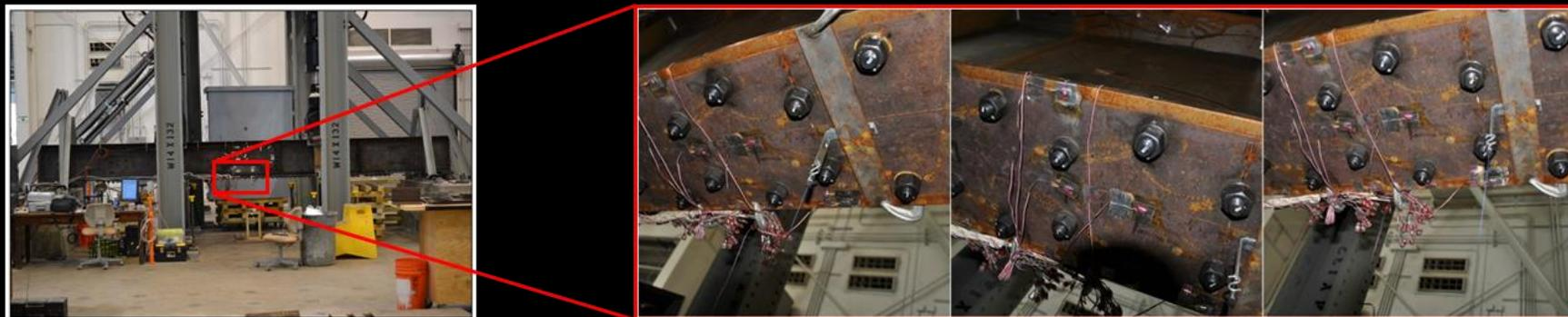
Fatigue testing on a steel girder (courtesy of Matthew H. Hebdon)
