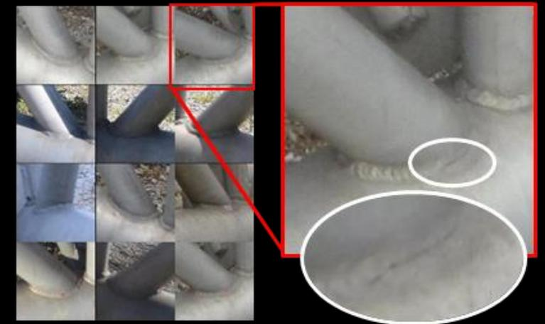
(f) Step 5: Damage detection
