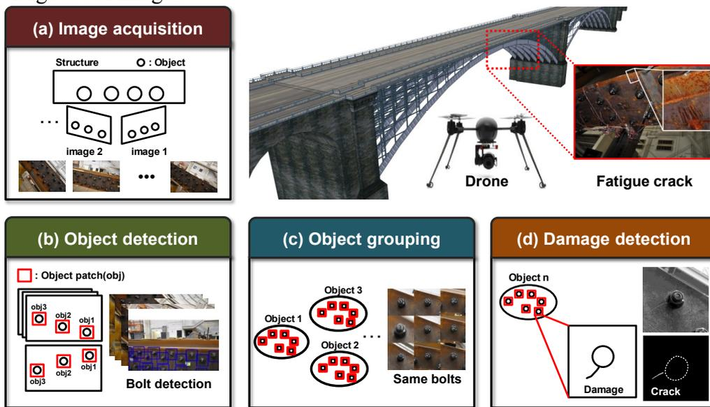
**Figure 2.** Steps in the proposed automated visual inspection technique
