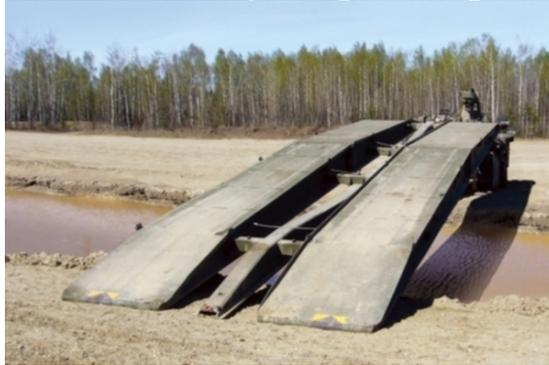
**Figure 4.** A typical mobile bridge (General Dynamics, 2015)
