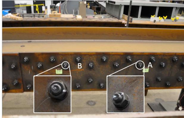
**Figure 3.** Specimen: a rusty, steel beam with 68 near identical bolts
