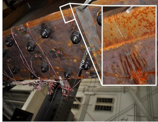
Images of a fatigue crack from different view points
