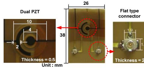
Figure 4. The dimension of the new dual PZT with flat type connectors used in this study
