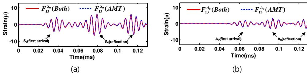
Figure 2. Comparison decomposed  $S_0$  and  $A_0$  mode signals using the collocated dual PZTs for selective generation denoted ‘Both’ to the proposed amplitude matching technique denoted ‘AMT’: (a)  $S_0$  mode (b)  $A_0$  mode (‘Both’ indicates that a selective mode can be generated by using collocated dual PZTs. ‘AMT’ means the signal decomposition based on the proposed amplitude matching
