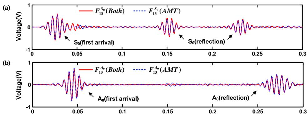
Figure 5. Comparison decomposed  $S_0$  and  $A_0$  mode signals using the collocated dual PZTs for selective generation denoted ‘Both’ to the proposed amplitude
