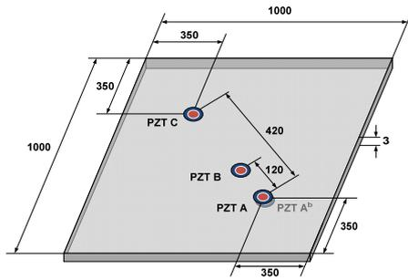
Figure 3. The configuration and size of the test specimen including four dual PZTs
